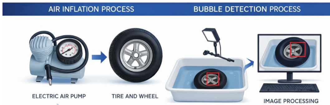
Figure 1. Experimental setup for tire leak detection consisting of two stages: air inflation using an electric pump and bubble detection via water immersion and vision-based image processing. Leakage is identified from bubble formation captured by a camera and analyzed digitally.
