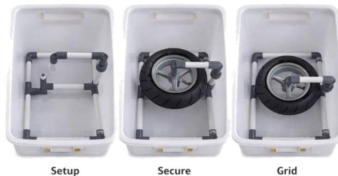
Figure 3. Assembly stages of the tire immersion test fixture. From left to right: (a) initial setup of the PVC support frame inside the water container, (b) placement of the tire and wheel assembly onto the support structure, and (c) final secured configuration prior to leak testing. The fixture ensures stable positioning and consistent immersion conditions during bubble-based leak detection experiments.
