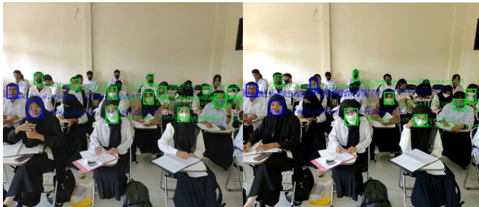
Figure 5 The proposed system's testing successfully detected WM (wearing masks) and NWM (not wearing masks/unmasked) student objects in the classroom
