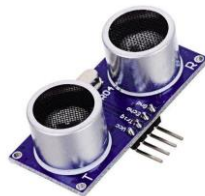
Figure 3. HC-SR04 (Ultrasonic Sensor)
